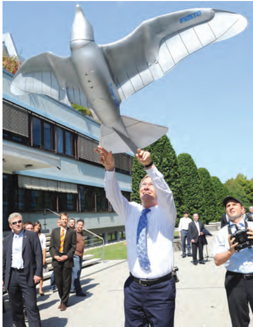
^ The 2-meter wide SmartBird drone was modeled after a herring gull.
